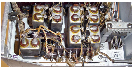
The bank of 0.5 mfd paper bathtub capacitors. After doing some testing, I'm hoping that all might still be ok.
