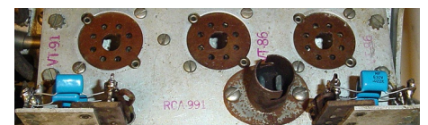
The r.f. and converter tube shelf with six new capacitors (three on each side) installed on the old terminal lugs.
