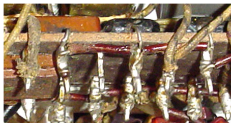
Inaccessible capacitors (top part of picture) were removed from the circuit by cutting their leads where they wrapped around the top of the resistor board. This made it possible to install new caps on the other side of the board (see text).
