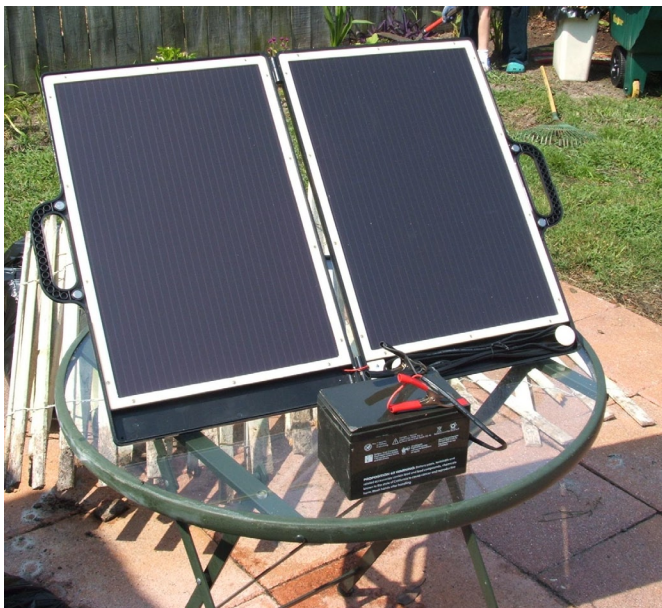
Solar panels connected to charge a 12 volt battery can be used to provide power to radios in an emergency
