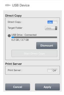
**3** When the completion message is displayed, unplug the USB device and tap *OK*.
