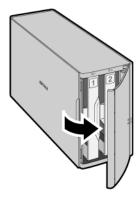
**3** Push the failed drive's cartridge up and remove it from the LinkStation.
