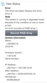
3 Check the status of the drive that failed. Follow the instructions to shut down the LinkStation.
