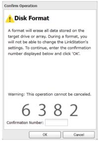
**6** Depending on the size of your drive, the format may take several minutes to several hours to complete. The power LED will flash during the format. Shared folders cannot be accessed during a format. Do not turn off the LinkStation until the disk format is finished.
