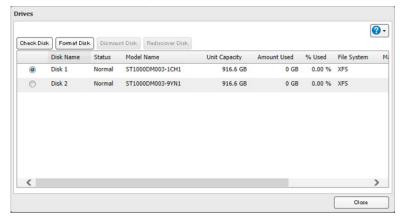
**Note:** If you connect an external drive to the LinkStation and the drive status is still shown as "Unformatted", refresh the status by clicking *Rediscover Disk*. If the status doesn't change, disconnect and reconnect the USB drive.
