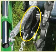
A torsional dampening spring (highlighted) allows the rake wheels to float more freely for smoother raking.
