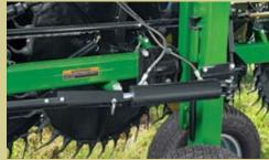
The rake beams on the WR5417 can be locked for easy transport and storage.
