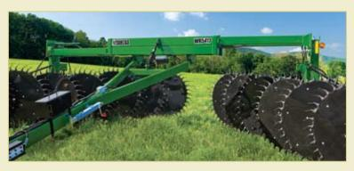
The WR5417 offers a maximum raking width of 29 feet for wider coverage. Or if your operation calls for one-sided raking, the rake wheel beams can be angled independently to the desired position. Hydraulically adjust your windrow width from 24 inches to 72 inches from the seat of your tractor.
