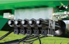
Make a variety of rake adjustments – like windrow or transport width – all from your tractor seat by using just one hydraulic remote (not shown) to activate the switches on the rake's electric control box (left). The control box connects to the rake's hydraulic valve bank to activate all of the cylinders (right).
