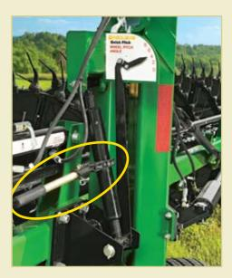
The rake beams on the Frontier Heavy-Duty Wheel Rake feature variable adjustment for setting the wheel straight or tilted based on an 8-degree of difference. Decrease angle to minimize debris pickup, or increase angle when gathering wet hay. Use the ratchet handle (highlighted) to adjust tilt angle. The handy meter lets you know when you're at your desired angle.
