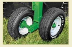
Tandem wheels provide smooth level raking when working over uneven terrain and contours.
