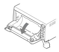
Remove the sheet from the leading edge of the paper, pull out about 15 cm (6 in.) of the paper, and then set the paper roll in the paper tray.
