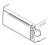
**2** Press the OPEN button to open the door.
