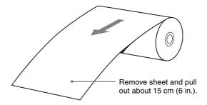
Load the paper with the printing side (heat sensitive side) up. Printing is not possible if the paper is reversed.
