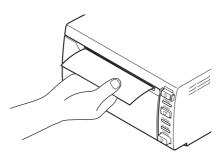
Clean the platen roller using a soft cloth moistened with ethyl alcohol when it becomes dirty.
