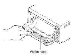
Press and hold down the FEED button so that the platen roller turns automatically. Release the FEED button when the surface of the platen roller to be cleaned appears.
