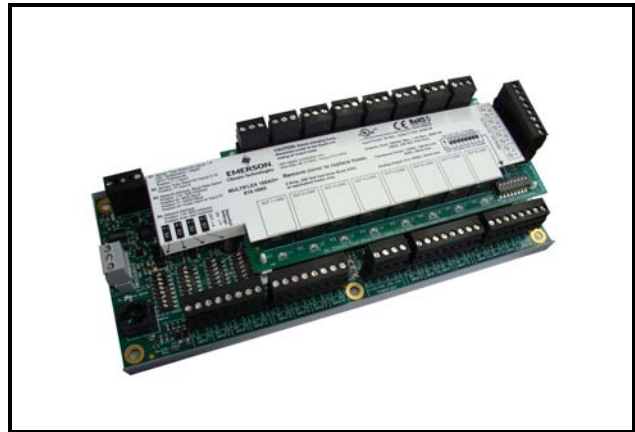
Figure 2-4 - RoHS MultiFlex Combination Input/Output Board (Side View)
