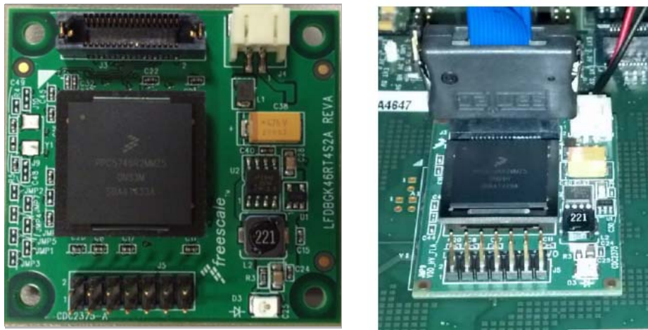
Figure 19. 292 BGA to 252 PGA Adapter card for Emulation and Debug Device
