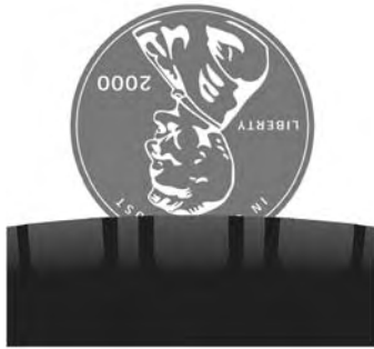
Exposed tread bars (replace)
