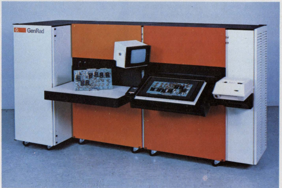
Four-line scanning increases the accuracy of GenRad's 2270 in-circuit tester. Bar-graph displays on the CRT ease potentiometer presetting and trimming.
