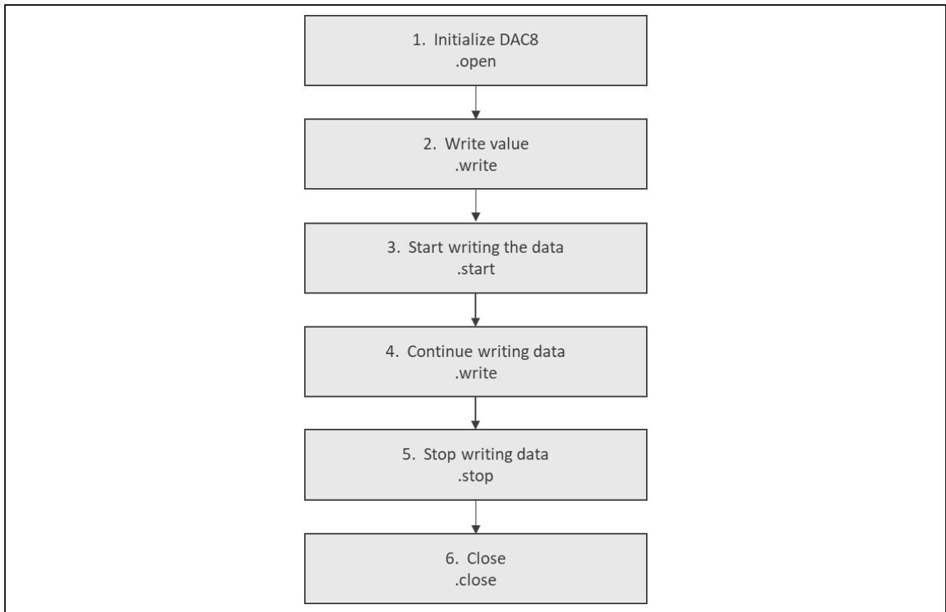
Figure 3 Typical DAC8 HAL Module Application Flow Diagram
