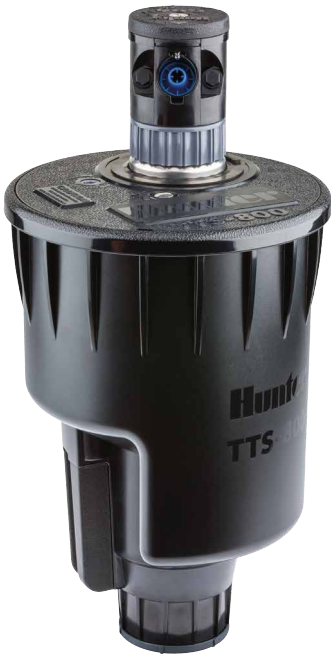
TTS-884 Pop-up height: 9.5 cm Overall height: 30 cm Flange diameter: 18 cm Female inlet: 1½" (40 mm) Acme
