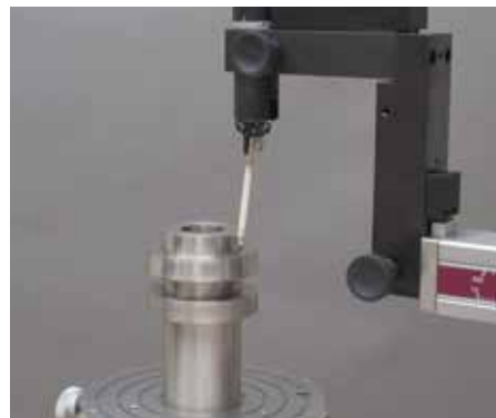
Spiral-mode cylinder measurement
