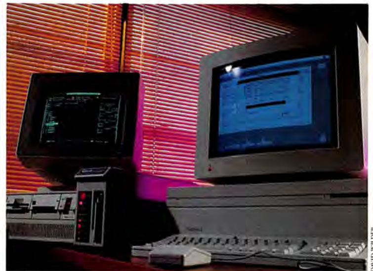
Tecmar's NuLink System allows Mac IIs and IBM PCs and PS/2s to share cartridge tape drives.
