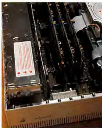
This series of modem boards in the Mac II lets the II work as a network modem-server.
