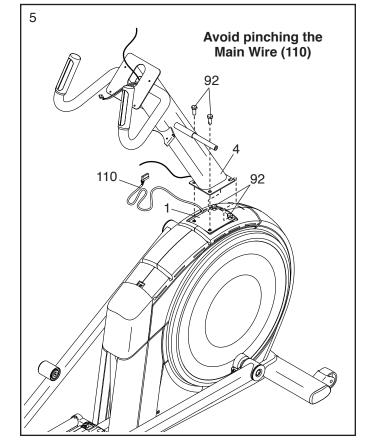
Locate the wire tie (A) in the lower end of the Upright (4). Tie the wire tie to the Main Wire (110) as shown. Then, pull the upper end of the wire tie until the Main Wire is routed through the Upright.
