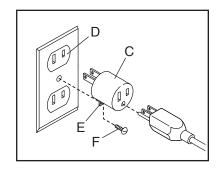
The lug (E) or wire extending from the adapter must be connected with a metal screw (F) to a permanent ground such as a properly grounded outlet box cover. Some 2-pole receptacle outlet box covers are not grounded. Before using an adapter, contact a qualified electrician to determine whether the outlet box cover is grounded before using an adapter. The temporary adapter should be used only until a properly grounded outlet can be installed by a qualified electrician.
