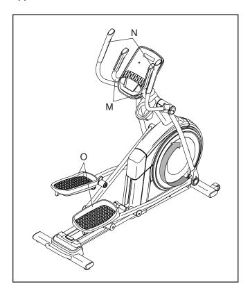
To dismount the elliptical, wait until the pedals (O) come to a complete stop. Note: The elliptical does not have a free wheel; the pedals will continue to move until the flywheel stops. When the pedals are stationary, step off the higher pedal first. Then, step off the lower pedal.
