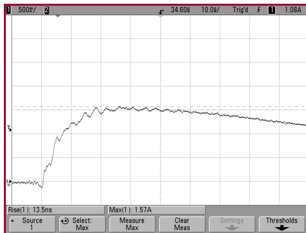
Figure 5.0-7: Current waveform through a 500 Ohm resistor at 4000V
