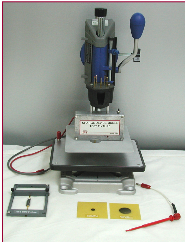
Figure 6.0-4: Model 9903 Charge Device Model Test Fixture
