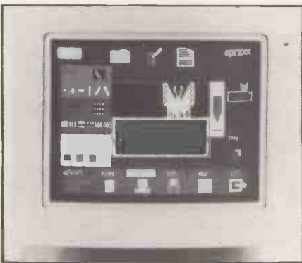
The icon editor uses Macpaint-like techniques, with various colours and stipples available.
