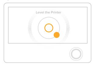
It is important the printer sits level so that resin does not overflow from the tank during printing.
