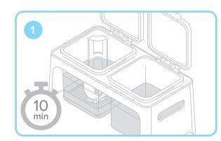
Drop your print in the rinse bucket and leave for 10 minutes. Agitate the part and repeat with the second rinse bucket. This two step process will help your IPA last longer.
