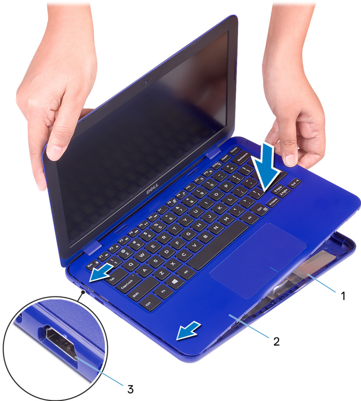
Figure 8. Replacing the base cover
