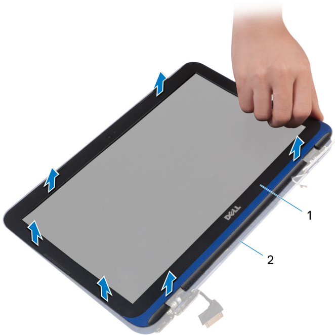
Figure 33. Removing display bezel
