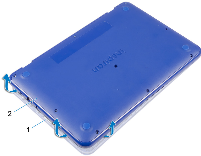
Figure 4. Removing the base cover
