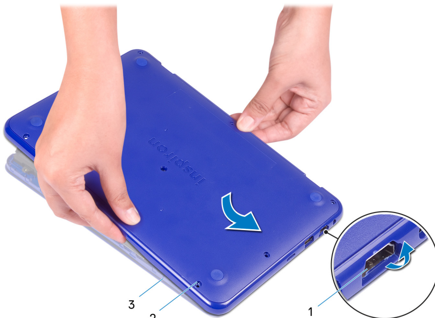
Figure 5. Removing the base cover
