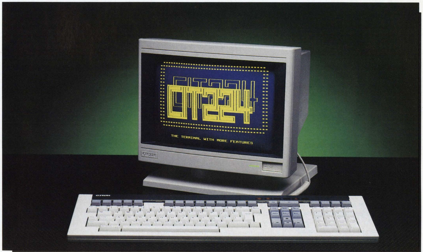
The CIT-224 terminal emulates a DEC VT220, VT100 or a VT52.
