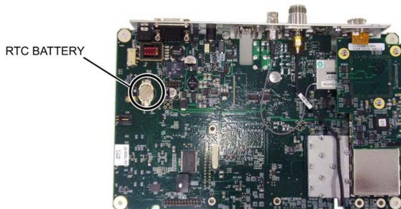
Figure 3-6. RTC Battery Location
