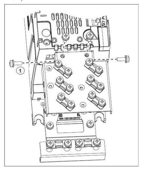
3. Remove outer insulation of the cable at the cable clamp and ground the bare shield under the clamp (2). Use a tightening torque of 1.5 Nm (13 lbf·in).
