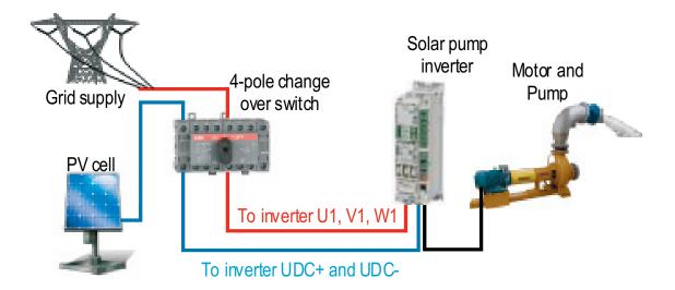
**Note**: Use two poles of the changeover switch in series to ensure that the voltage applied across each pole is half of the full DC voltage.
