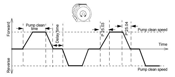
The cleaning sequence can be activated only in the manual mode of operation. The cleaning sequence starts in the forward direction and follows the reverse direction. This cycle repeats three times. If any intermediate fault occurs, the pump cleaning function stops.
