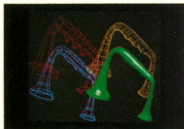
Bi-cubic surface control points, patches, polygon subdivision and shaded display: less than 3 seconds.
