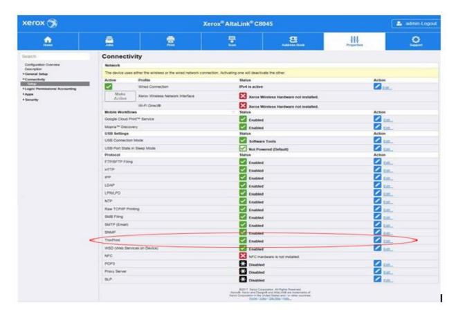
Once the ThinPrint Protocol is enabled the Admin has access to the settings below. The port must be enabled. The default port number for ThinPrint communication is 4000.
