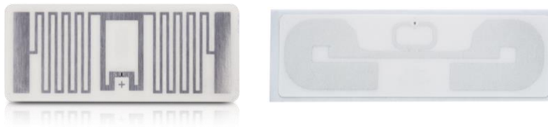
Example of clear and white RAIN UHF labels
