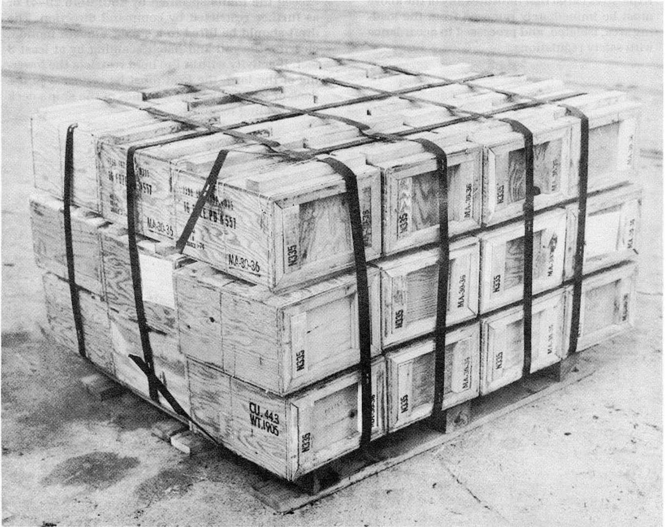
Figure 42. Unit load isolated because of defective banding.
