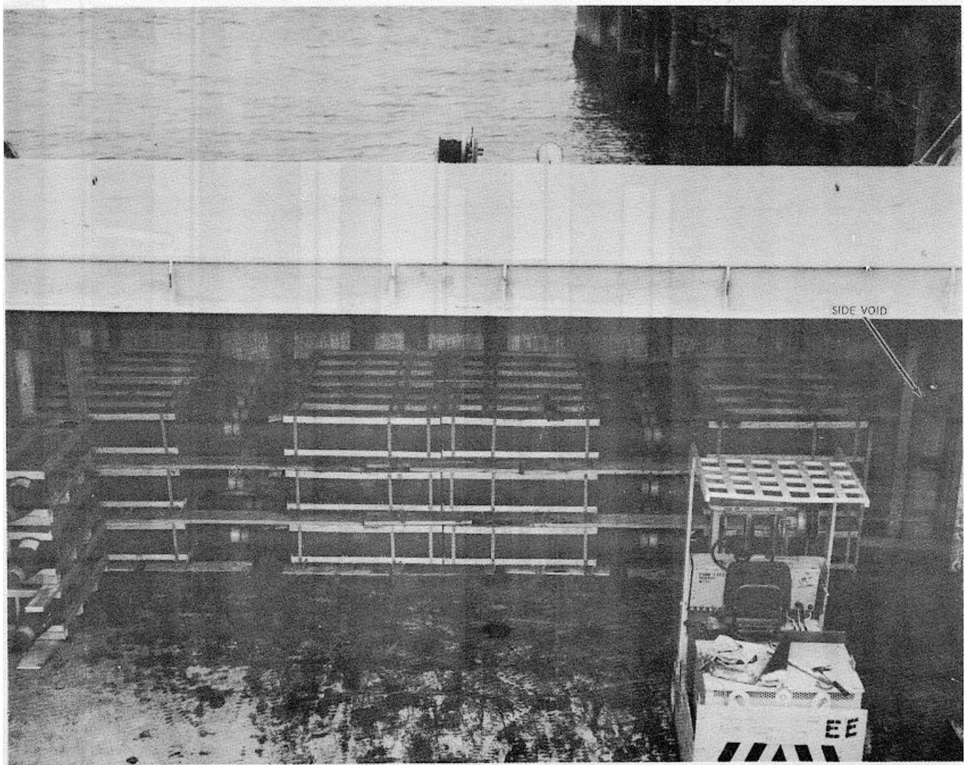
Figure 10-7. Staggered block stow of 1,000-pound-bomb unit loads, MK 83.
