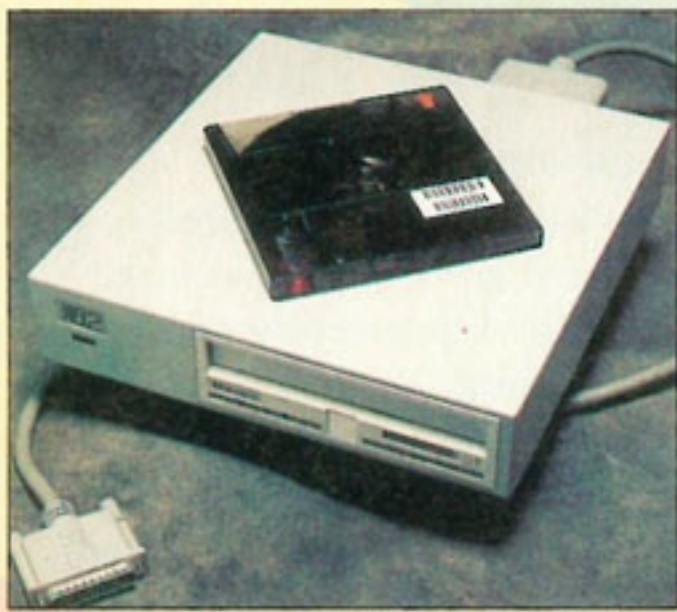
Above left is a typical SyQuest removable drive – this one is made by d2 Systems. Each cartridge can store around 40Mb of data. On the right is a Mac's internal hard drive – this one is an 80Mb unit, manufactured by IBM
