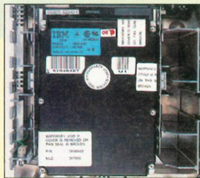
Above left is a typical SyQuest removable drive – this one is made by d2 Systems. Each cartridge can store around 40Mb of data. On the right is a Mac's internal hard drive – this one is an 80Mb unit, manufactured by IBM
