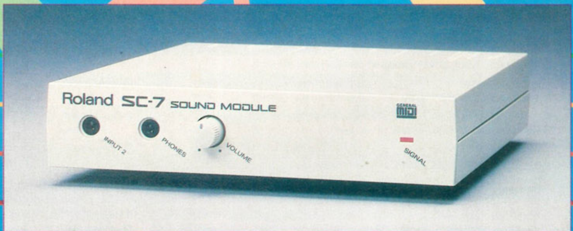
And above we have the third component of the Roland system – the SC-7 sound module which contains the MIDI interface which hooks up to your Mac. You just plug the keyboard in, load up some software and ta da da... ....you're jamming, illing and kicking 'til ya dropping!
