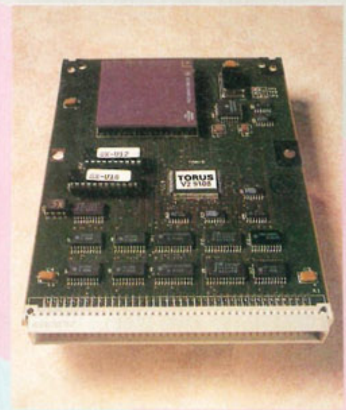
This is a TokaMac accelerator. The large grey object is the 68040 processor
