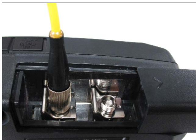
Figure 2.6-1 Connecting Fiber to Measurement Port
