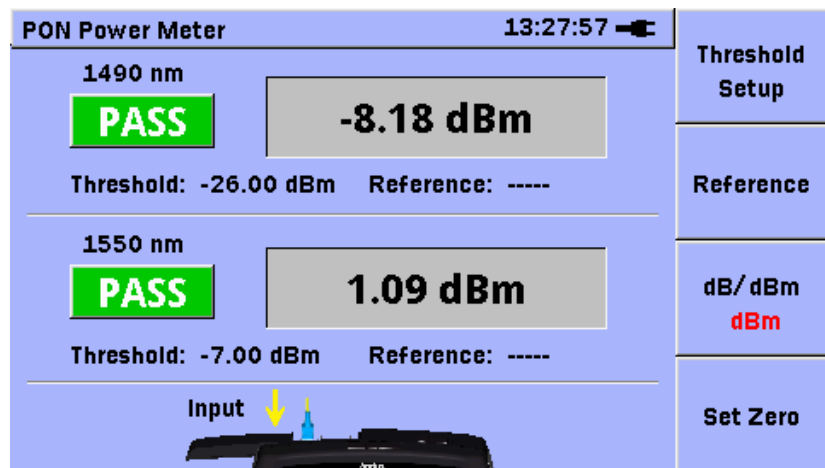
Figure 1.1.5-1 PON Power Meter Screen
