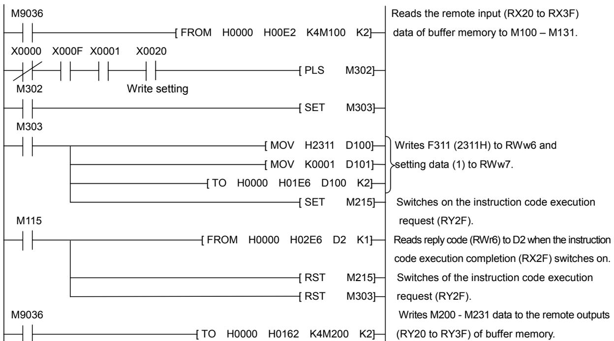
\*To write parameters, add the triple figures that follow Fxx to 2000H.
