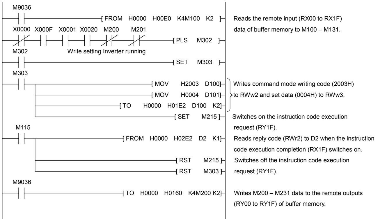
Stores reply code to D2 when the instruction code execution completion.
