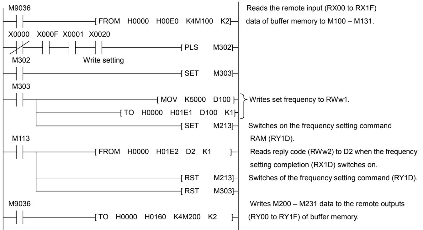
\*To continuously change the running frequency from the PLC
