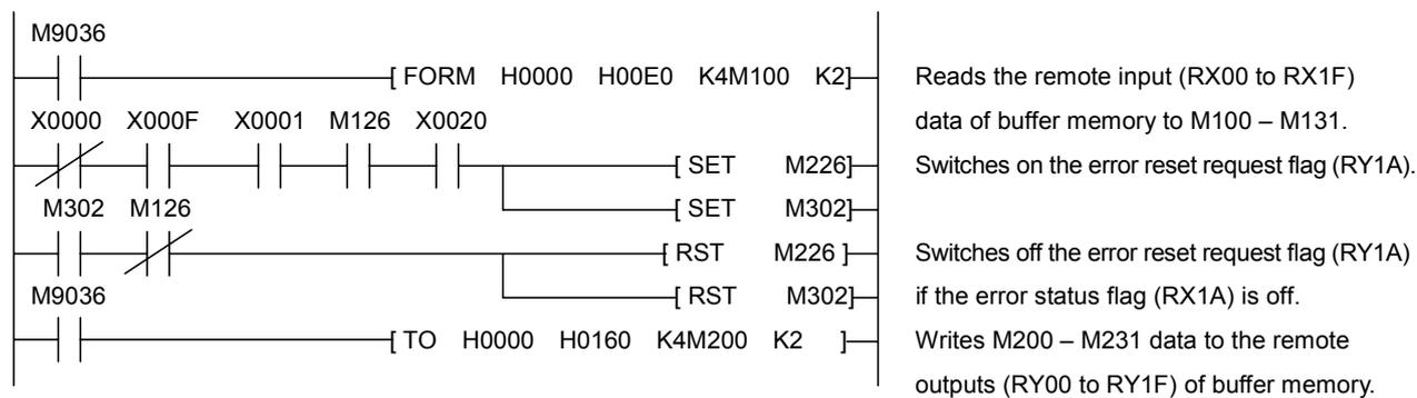
\*The above inverter reset using RY1A may be made only when an inverter fault occurs.
