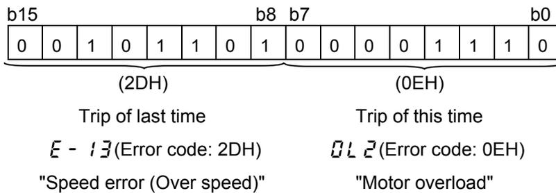
\*For details of error code, refer to "Section 4.4.4. The details of an error code".
