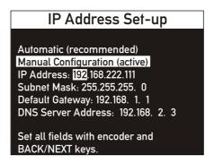
Changes are saved automatically – exit by either pressing MENU to drop back through the levels or power/home to get back to the home screen. Note that the manual IP address will not be shown on the home screen until a valid network connection is established (CTRL LED is illuminated).
