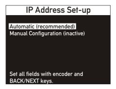
To change this to manual, press NEXT to display all the manual set-up parameters.
