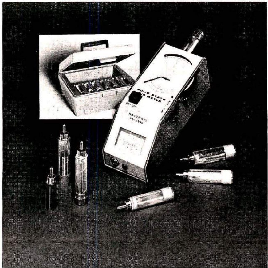
For those who can use a transmitter to help in determining the performance of an antenna an swr meter is a valuable tool. Experimenters without transmitters will have to use other methods, such as the grid-dip meter shown here.
