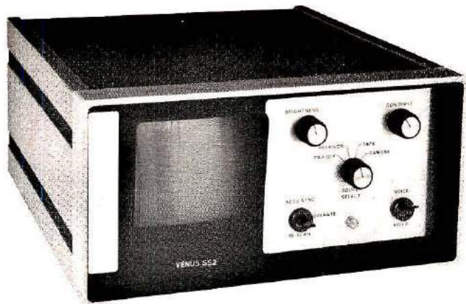
Fig. 1. If you are looking for SSTV monitors, you might find a Robot like this early Model 70, shown here with matching camera. Later versions would be 70A, B, or C. All are good buys for the newcomer if you can find one secondhand. The Venus Scientific SS-2 Monitor at the right also has a P-7 phosphor and is a good unit either assembled or as a kit.
