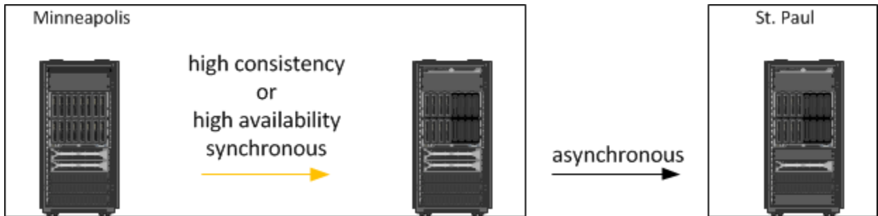
Figure 27 Intra campus and metro DR sites – Cascade topology – fibre channel and iSCSI replication
