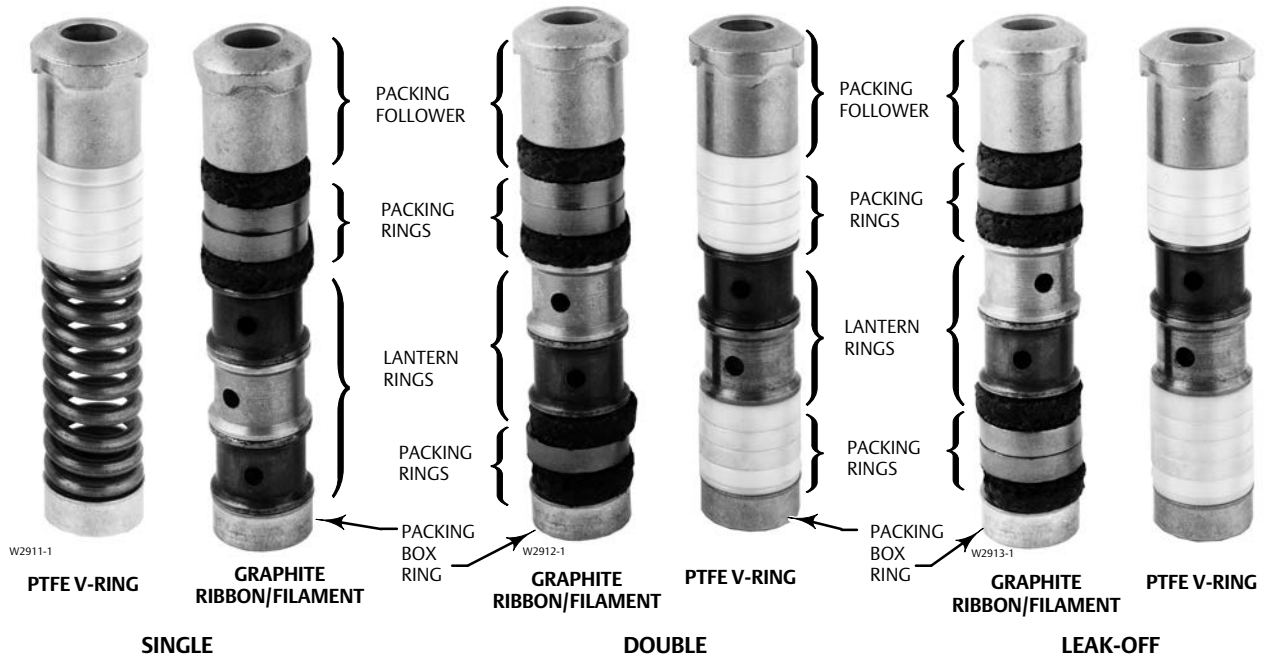
Typical Packing Arrangements. For Packing Arrangement Cutaway Drawings, see figures 1, 2, 3, 4, 5, 6, 7, and 8.
