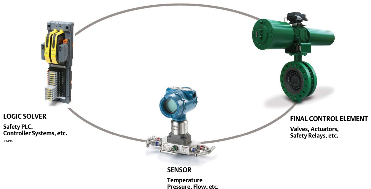
Figure 2. Components of a Safety Instrumented System
