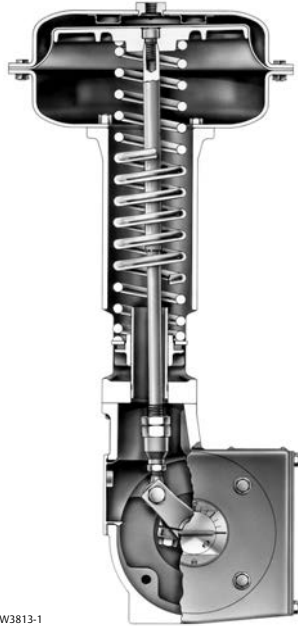
Figure 2. Sectional Views Typical of 1052 Actuator
