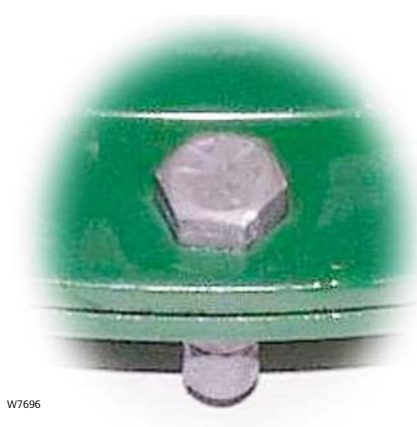
Powder-Coated Actuator Casings with NCF Coated Cap Screws after 500 Hours in an Accelerated Salt Spray Laboratory Test
