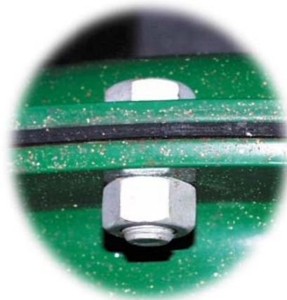
Powder-Coated Actuator Casings with NCF Coated Cap Screws after One Year of Service on an Off-Shore Platform (Light-Colored Spots are Paint Drift from Customer Paint Spraying of Nearby Equipment)
