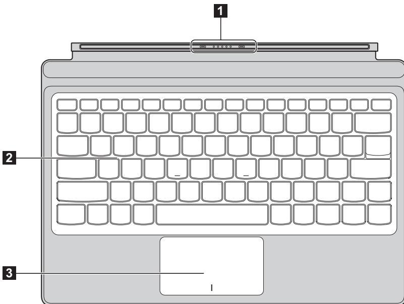
**1 Pogo pin with guide pin** Connect the tablet to the keyboard Folio and secure it in the installation position.
