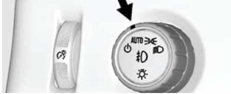
Exterior Lamp Controls here
