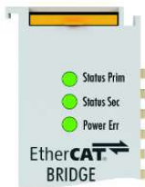
Fig. 191: The operating state is indicated via diagnostic LEDs
