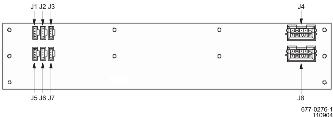
Figure 110-3. Fan Tray Front Panel Connectors (Rear View)
