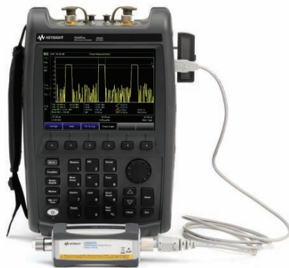
Keysight's FieldFox pulse measurements simplify radar field testing.
