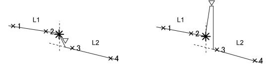
Figure 3.6.4-1 Method to Obtain Splice Point Loss
