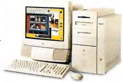
Apple's Power Macintosh 9600/350 uses the 350-MHz 604e CPU.
