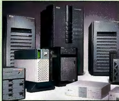
Sun's Enterprise 450 has 10 PCI slots, including 66-MHz, 64-bit-wide ones.
