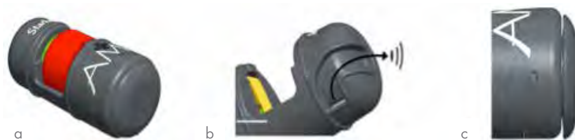
Figure 2: Three innovative design features of AMP. (a) represents the circular cross section with no sharp corner transitions. (b) represents the five-mm long acoustic channel leading from the receiver. (c) shows the 360° sound inlet port to the microphone.
