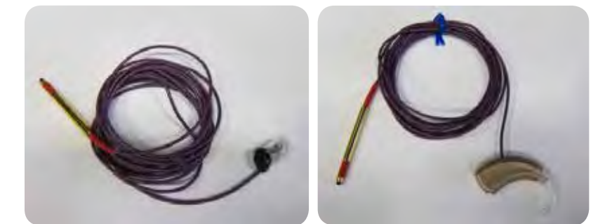
Figure 2. IIC and BTE hearing aids are shown. Each was specially prepared for recording; a cable has been attached to the hearing aid microphone for in situ audio recording.
