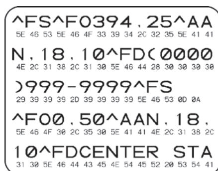
Figure 4 Communications Diagnostics Test Label
