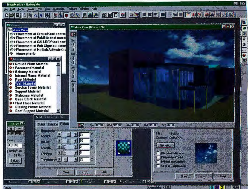
RealiMation supports multiple cameras, which you can instruct to travel through a virtual scene on preset trajectories.
