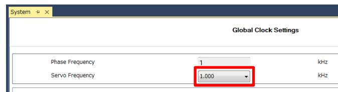
\* Servo Frequency is set to 1 kHz for the example in this document.
