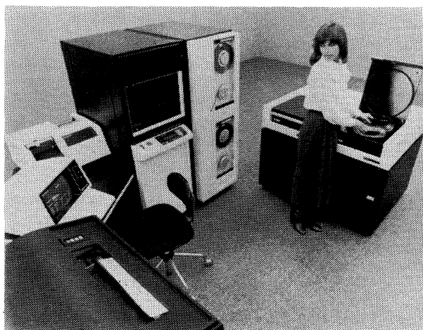
Honeywell's powerful new Level 6 Model 47 minicomputer can provide up to 2 million bytes of main memory and can process COBOL programs seven times faster than the earlier Model 33. The configuration shown includes (left to right) a 900-lpm printer, VIP 7200 console display/keyboard, 500-cpm card reader, CPU with 320K bytes of memory, two diskette units above the processor, two magnetic tape units, and two 256-megabyte disk units. Prices for the Model 47 begin at $28,050.
