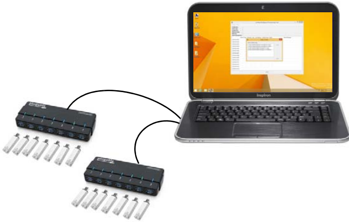
Figure 2-2: Provisioning multiple devices
