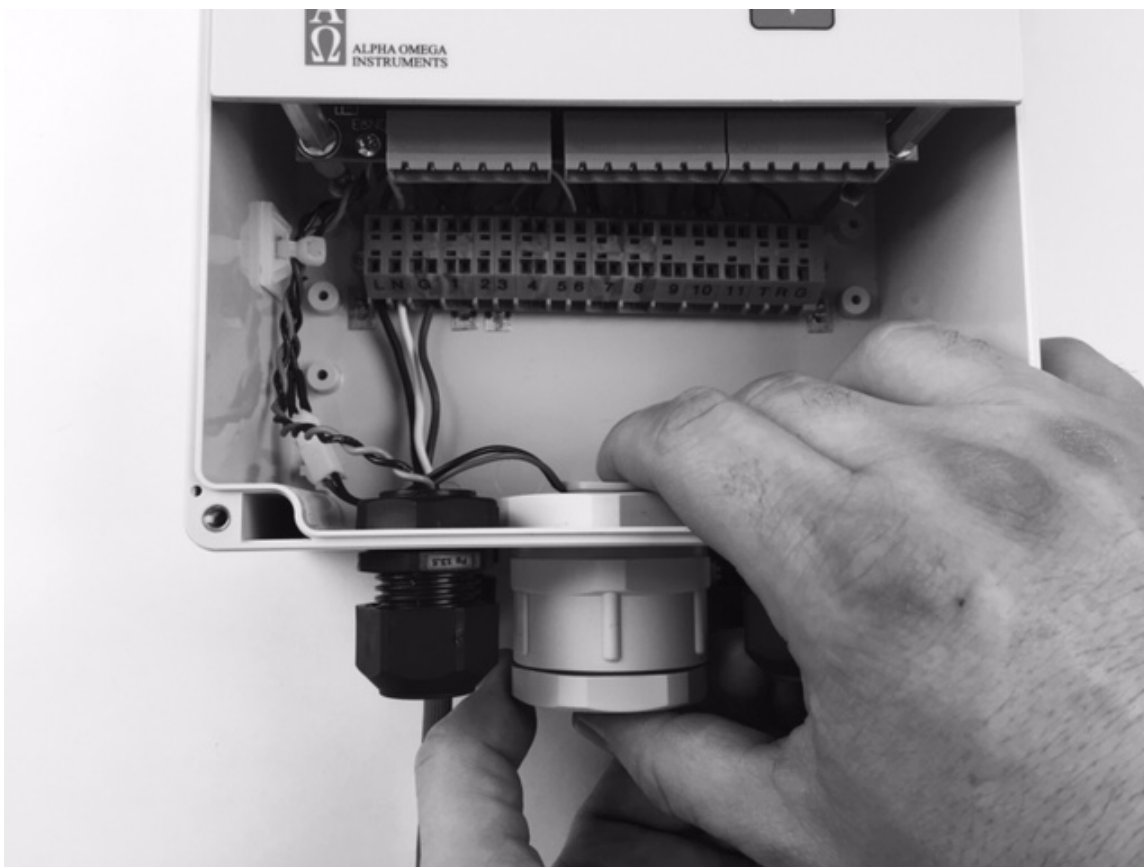
Figure 7 - Local Oxygen Sensor Installation
