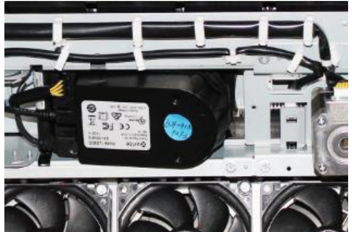
The X-Rite® Inline Spectrophotometer automates the collection of XRG data for calibration and profiling.
