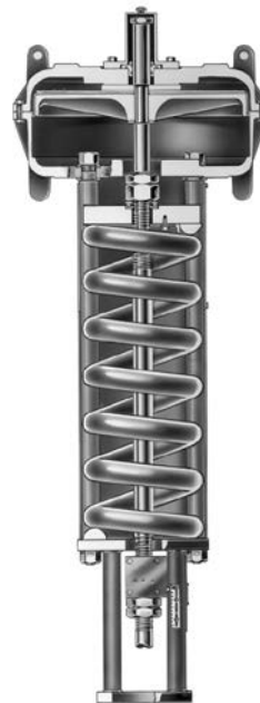
Figure 1. Sectional view of Fisher 657 Size 100 Actuator
