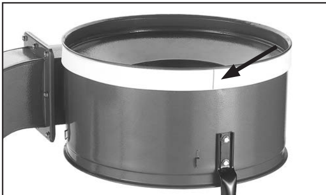
Figure 20. Trimmed foam strip.
