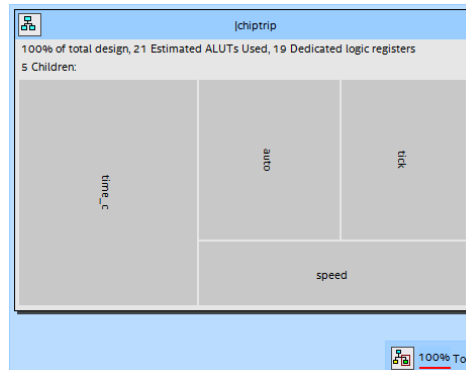
Figure 65. Top-Level Entity in the Design Partition Planner
