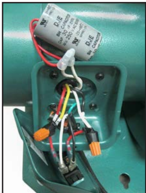
Figure 31. 120V junction box.
